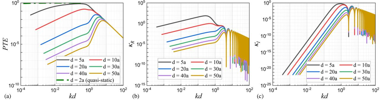
FIG. 8. Coplanar arrangement: a)  $PTE$  versus  $kd$ ; b)  $\kappa_R$  versus  $kd$ ; c)  $\kappa_I$  versus  $kd$  for different values  $d/a$  from 5 to 50.
