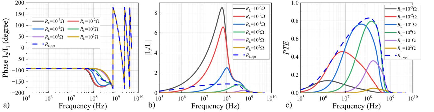
FIG. 5. Mid-range coupling between two lossy loops: a) phase difference between the loop currents; b) magnitude of the currents ratio  $I_2/I_1$ ; c) PTE for different values of the load resistance  $R_L$ . The dashed curves correspond to the optimal resistance, maximizing PTE.
