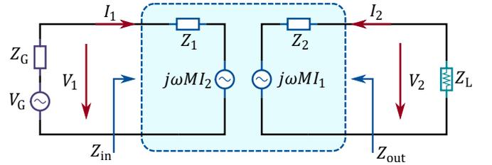
FIG. 1. Equivalent circuit model of the WPT system.
