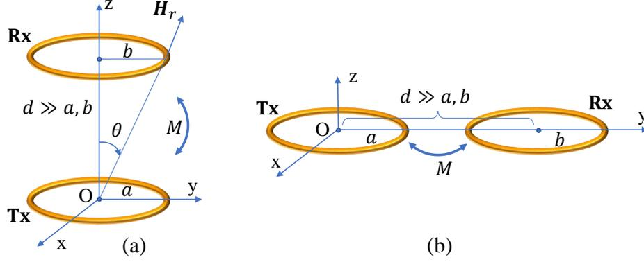
FIG. 2. Two magnetic dipoles in two case studies: a) coaxial position; b) coplanar position.
