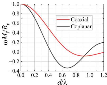
FIG. 3. Ratio of the mutual resistance to the radiation resistance for coaxial and coplanar arrangements of the Tx and Rx loops versus the normalized distance  $d/\lambda$  between the loop centers.
