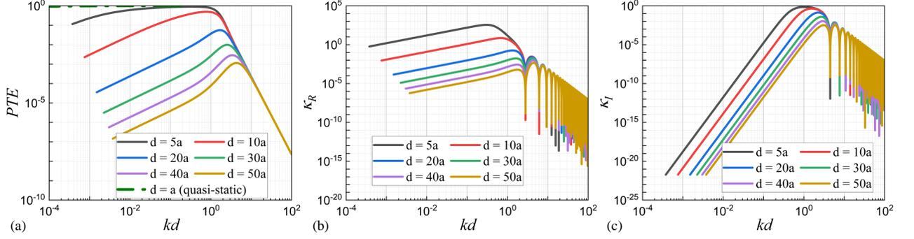
FIG. 7. Coaxial arrangement: a)  $PTE$  versus  $kd$ ; b)  $\kappa_R$  versus  $kd$ ; c)  $\kappa_I$  versus  $kd$  for different values  $d/a$  from 5 to 50.
