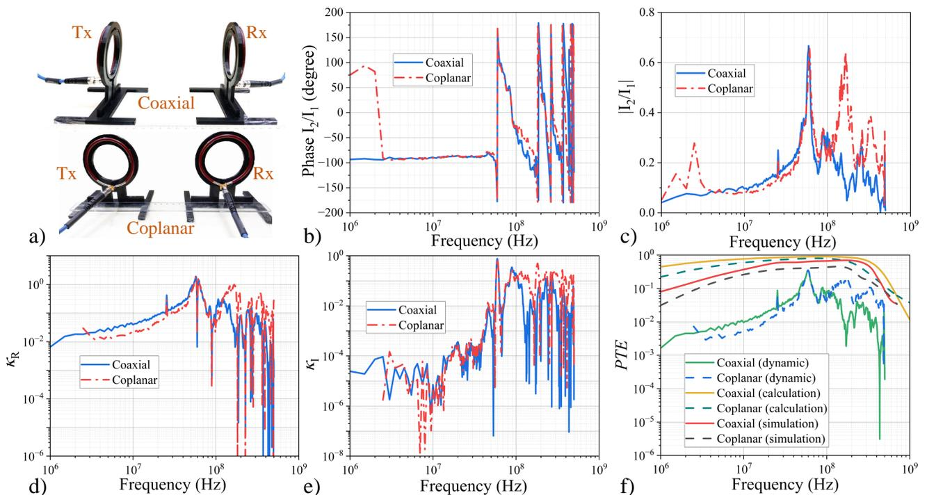
FIG. 11. Experimental setup and results: a) Two loop antennas in coaxial and coplanar arrangements; b) Phase difference of the loop currents; c) Magnitude ratio  $I_2/I_1$ ; d)  $\kappa_R$ ; e)  $\kappa_I$ ; f)  $PTE$  comparison between calculated, simulated, and measured results for coaxial and coplanar antenna arrangements.
