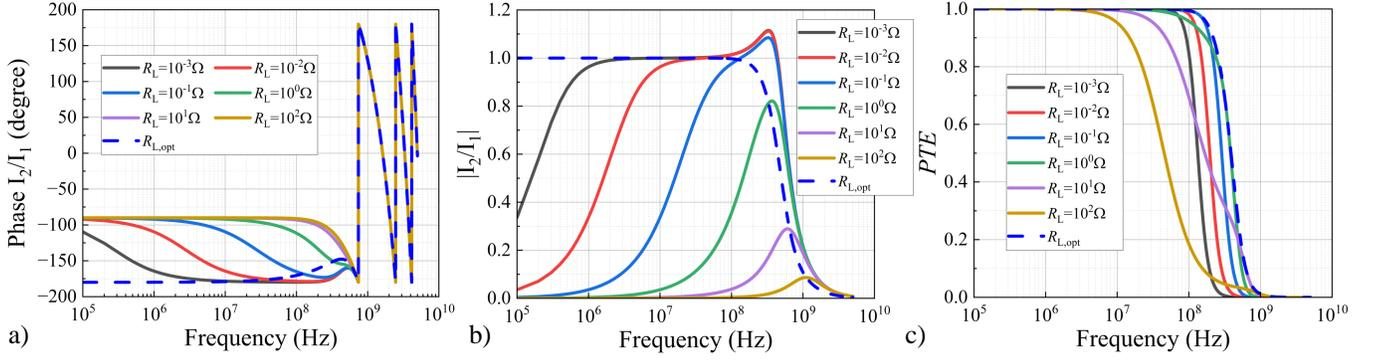
FIG. 4. Mid-range coupling between two lossless loops: a) phase difference between the loop currents; b) magnitude of the currents ratio  $I_2/I_1$ ; c) PTE for different values of the load resistance  $R_L$ . The dashed curves correspond to the optimal resistance, maximizing PTE.
