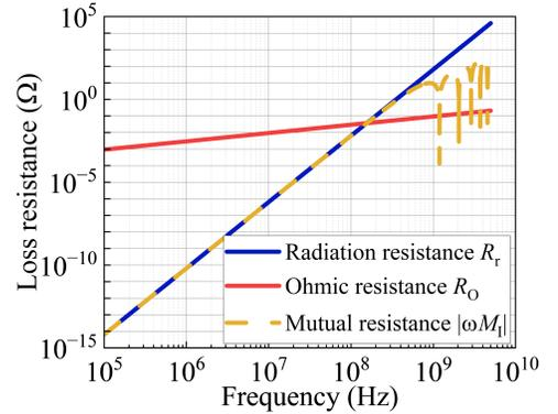
FIG. 6. Comparison of Ohmic resistance (19) and radiation resistances of one loop antenna (20), together with the mutual resistance between two antennas  $\omega M_I$ . The loop radius  $a = 36$  mm, and  $d = 5a$ .
