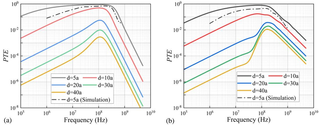
FIG. 9.  $PTE$  in a broad frequency range for different normalized transfer distances  $d/a$ . a) coaxial arrangement; b) coplanar arrangement.
