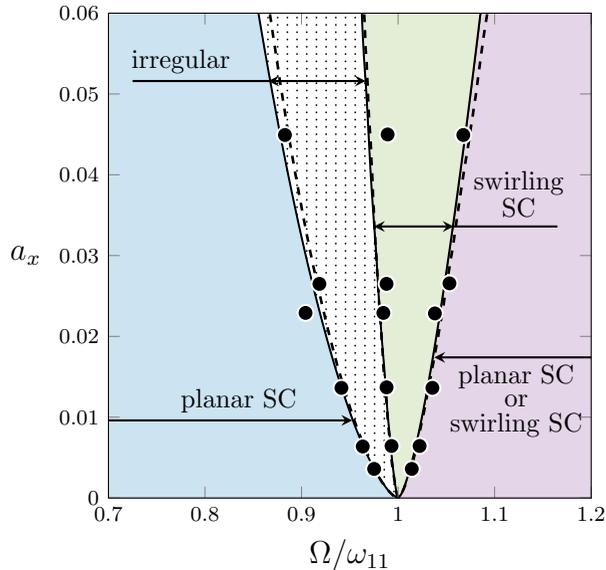
Figure 2: Estimates of bounds, in the  $(\Omega/\omega_{11}, a_x)$ -plane, between the frequency ranges where planar, irregular and swirling waves occur when the container undergoes a longitudinal and harmonic motion. Filled markers: experiments by Royon-Lebeaud *et al.* (2007). Black dashed lines: theoretical prediction by Faltinsen *et al.* (2016), whose theoretical curves have been here reproduced by manually sampling those reported in their original figure 8(a).
