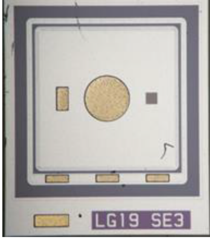
Figure 1: Photo of HPK device used in this work. The sensitive area is 1.3 \times 1.3 \text{ mm}^2 , active thickness is 50 \text{ }\mu\text{m} .
