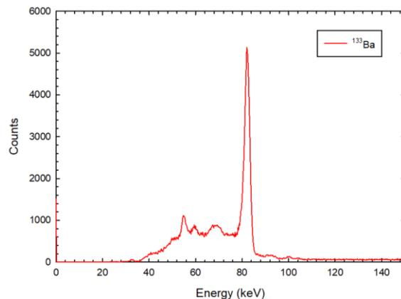
Fig. 11.  $^{133}\text{Ba}$  spectrum of all single events acquired with Caliste HD inside the tunnel at the LARIX facility.
