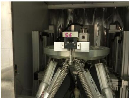
Fig. 15. Ge crystal grabbed by the hexapod available at LARIX to correctly orient each crystal tile to the proper Bragg's angle on the Laue Lens frame under the control of the X-ray pencil beam.
