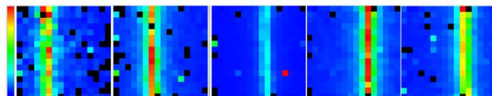
Fig. 20. Focal spot images acquired with the spectro-imager carrying out a fine scanning in the crystal central position in steps of 2 mm at 130 keV.
