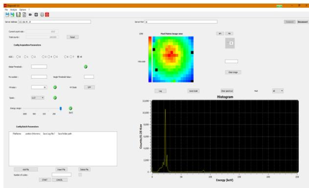
Fig. 6. Quick look and acquisition software supplied with the Wix camera by CEA.
