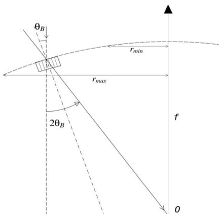
Fig. 1. Laue lens geometry.
