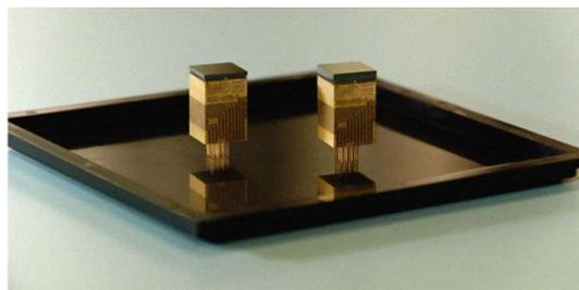
Fig. 3. Caliste HD detector module: the CdTe detector, manufactured by Acrorad (Japan), is bonded on top of it.
