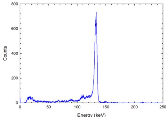
Fig. 18. Spectrum acquired with Caliste HD in the crystal central position at 130 keV. The result of the best fit is  $132.47 \pm 0.06$  keV.
