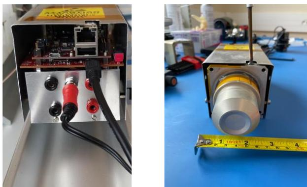
Fig. 5. Portable camera containing the CdTe detector and the related FEE. On the left, the connected Readout and thermoelectric coolers power cables are visible as well the Ethernet and Wi-Fi connectors. The copper tube ensures the hermeticity of the detector head (on the right) filled with Argon.
