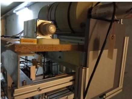
Fig. 14. Caliste HD in the focal plane position located at 11.5 m from the crystal close to the previous focal plane detectors.
