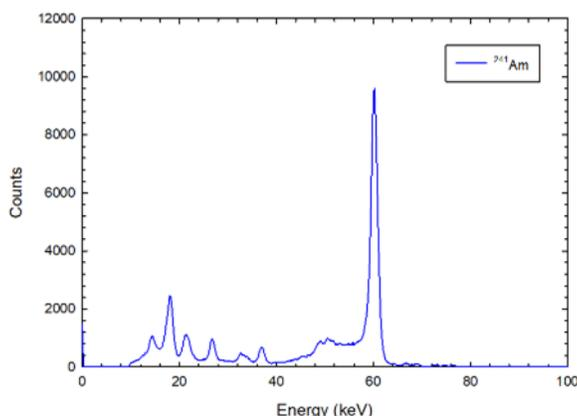
Fig. 10.  $^{241}\text{Am}$  spectrum of all single events acquired with Caliste HD at the Larix facility.
