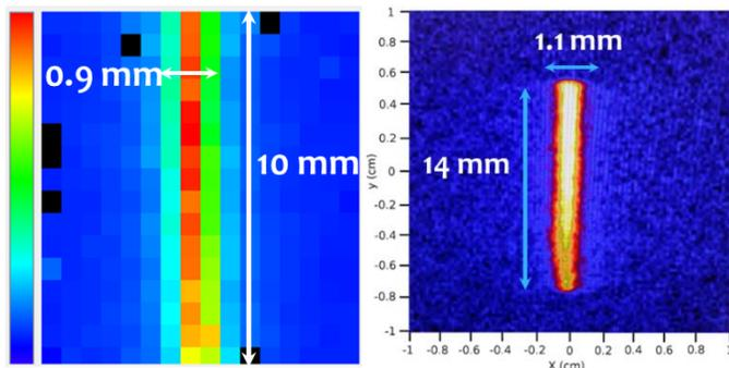
Fig. 17. Measured images with Caliste HD on the left and with the Perkin Elmer Flat Panel, based on a CsI(Tl) scintillator (0.8 mm thick), on the right.
