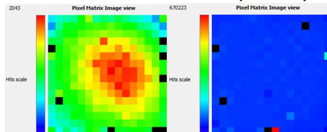
Fig. 12.  $^{109}\text{Cd}$  (left) and  $^{137}\text{Cs}$  (right) images acquired with Caliste HD at the OAS Bologna premises.
