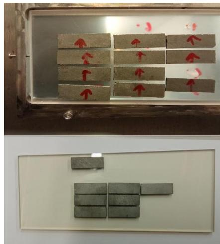
Fig. 22. The Laue lens prototypes are composed of 11 Ge crystals (top) and eight Ge tiles (bottom), each consisting of three rings.
