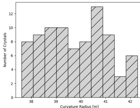
Fig. 16. Distribution of the curvature radius of 83 bent Ge (220) crystals.
