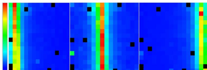
Fig. 19. Diffracted images of the focal spot acquired with Caliste HD in three crystal positions at 130 keV. The images are in focus but slightly shifted between them.
