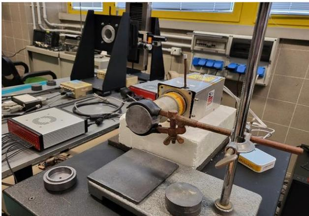
Fig. 4. Experimental setup available at the OAS Bologna premises. The radioactive source, contained in a Pb collimator placed in front of the radiation entrance window, is aligned to the detector with a laser. The detector window is made of 0.5 mm thick Al.
