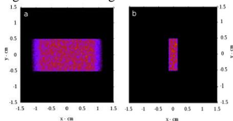
Fig. 2. Diffracted images obtained simulating a beam ( $20 \times 10 \text{ mm}^2$ ) incident on a mosaic (15 arcsec mosaicity) GaAs (220) crystal tile. The source of radiation is placed at an infinite distance from the target.
