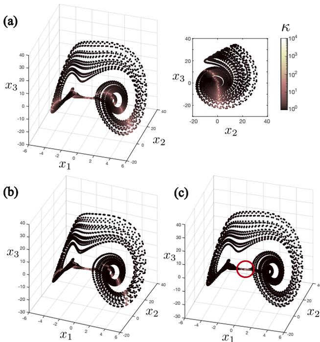
FIG. 7. Coefficient of (a) complete observability, (b) functional observability with respect to  $g_1(\mathbf{x})$ , and (c) functional observability with respect to  $g_2(\mathbf{x})$  computed over the state space of the Cord attractor.
