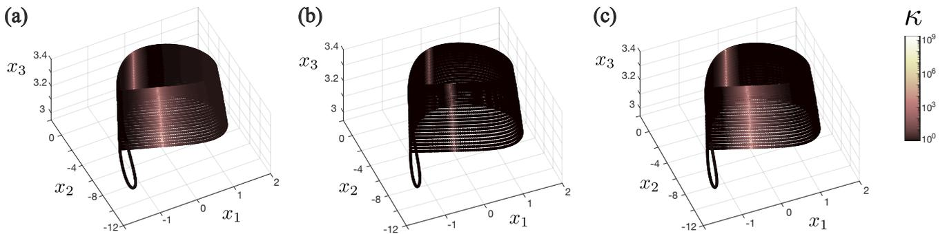
FIG. 8. Coefficients of (a) complete observability, (b) functional observability with respect to  $g_1(\mathbf{x})$ , and (c) functional observability with respect to  $g_2(\mathbf{x})$  computed over the state space of the HR neuron model, considering the measured time series  $y = h_2(\mathbf{x})$ . Simulations are presented for  $(T, T_{\text{trans}}) = (2500, 1500)$ .
