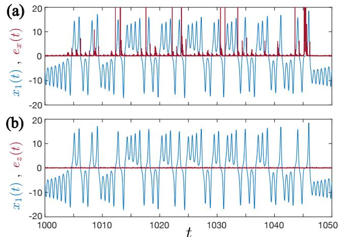
FIG. 4. Reconstruction error (red line) of the Lorenz system as a function of time for the (a) entire state vector  $\mathbf{x}(t)$  and (b) functional vector  $z(t) = x_1(t)$  sought to be reconstructed. Time series of  $x_1(t)$  (blue line) is shown for reference.
