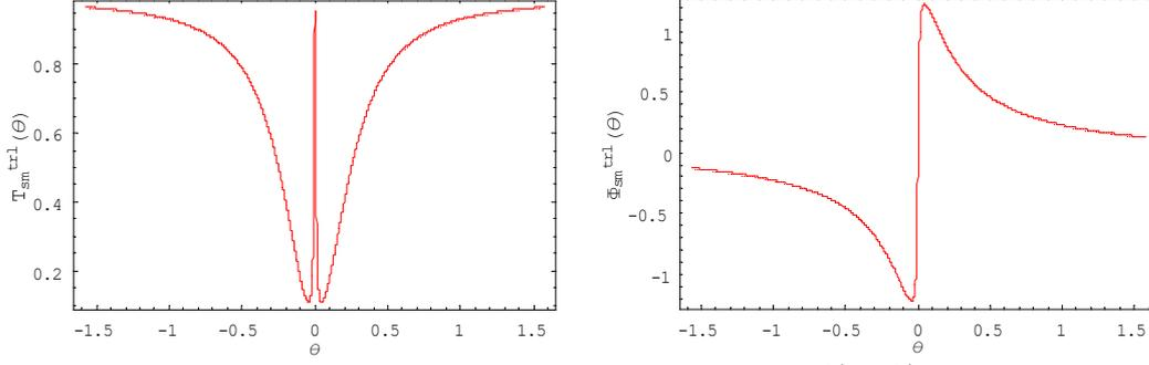
**Figure 5** The transmission and the phase shift spectra for  $T_{sm}^{tr1}$ ,  $\Phi_{sm}^{tr1}$  with parameters  $r_1 = 0.999$ ,  $r_2 = a_1 \times a_2$ ,  $a_1 = 0.9999$ ,  $a_2 = 0.88$  versus  $\theta$  in unit of radian.
