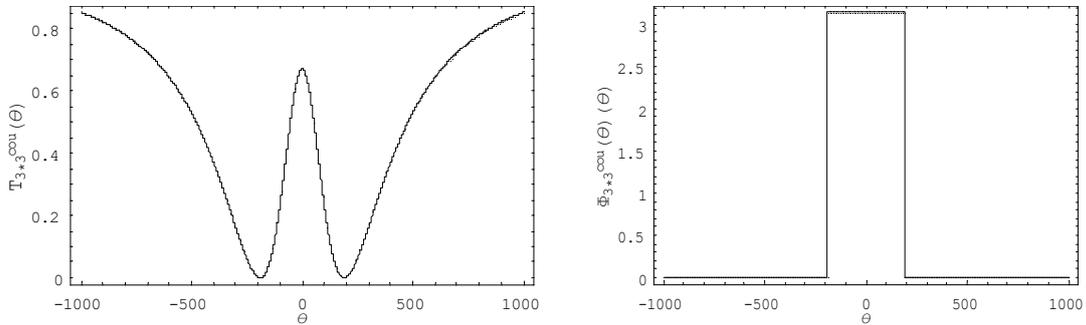
**Figure 9** The transmission and phase shift spectra for  $T_{3 \times 3}^{cou}$ ,  $\Phi_{3 \times 3}^{cou}$  with parameters  $t = 0.9998$ ,  $\alpha = 0.99998$ ,  $\mu = 0$ ,  $\delta = 0$  versus  $\theta$  in unit of  $10^{-4}$  radian.
