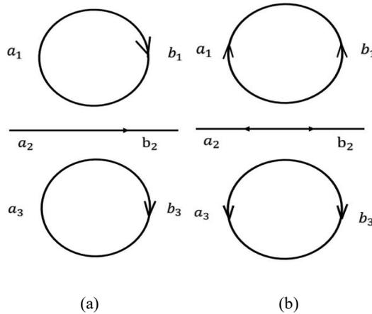
**Figure 7.** Schematic diagram of  $3 \times 3$  system, (a) the traveling wave coupling, (b) the counter-propagation waves coupling.
