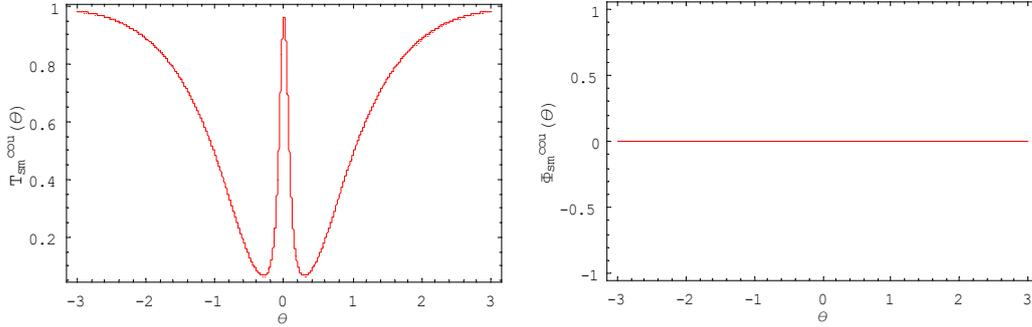
**Figure 6** The transmission and phase shift spectra for  $T_{sm}^{cou}$ ,  $\Phi_{sm}^{cou}$  with the parameters  $r_1 = 0.999$ ,  $r_2 = a_1 \times a_2$ ,  $a_1 = 0.9999$ ,  $a_2 = 0.88$  versus  $\theta$  in unit of radian.
