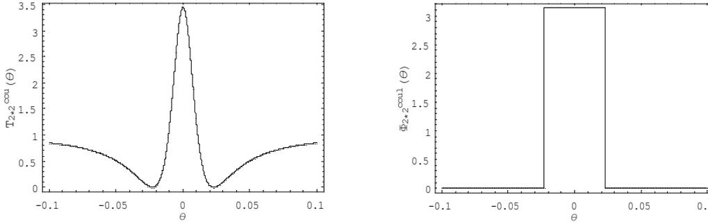
**Figure 4** The transmission and phase shift spectra with the parameters  $t = 0.9998$ ,  $\alpha = 1.00006$  versus  $\theta$  in unit of radian.
