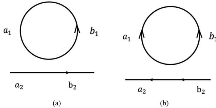
**Figure 1** Schematic diagram of  $2 \times 2$  system, (a) traveling wave coupling, (b) counter-propagating wave coupling.
