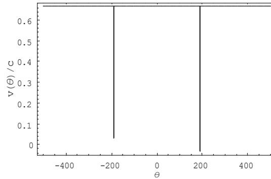
**Figure 10.** The phase velocity spectra for  $3 \times 3$  system versus  $\theta$  in unit of  $10^{-4}$  radian.
