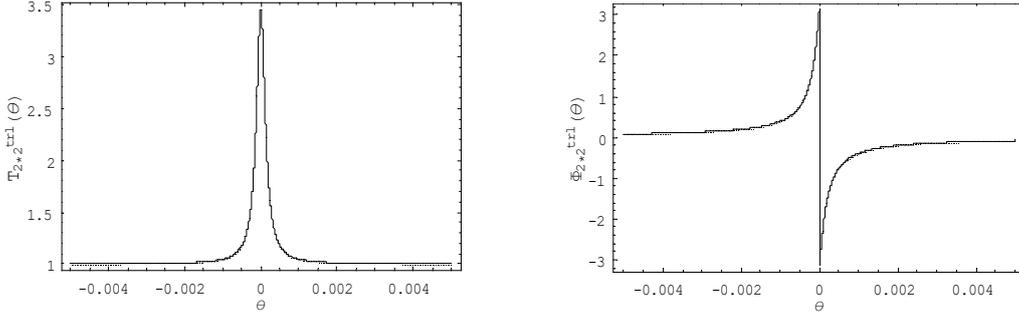
**Figure 3** The transmission and phase shift spectra with the parameters  $t = 0.9998$ ,  $\alpha = 1.00006$  versus  $\theta$  in unit of radian.
