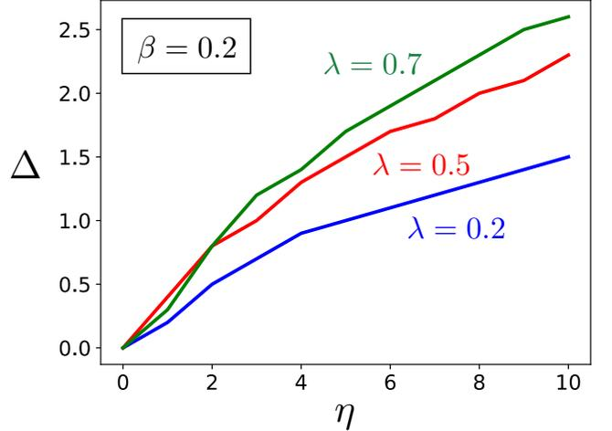
FIG. 7. Synchronization boundaries of two coupled quantum DvdP oscillators for different values of  $\lambda$ . Comparing with Fig.2b in the main text, we see that the additional Kerr nonlinearity  $\beta = 0.2$  does not change the synchronization boundary.
