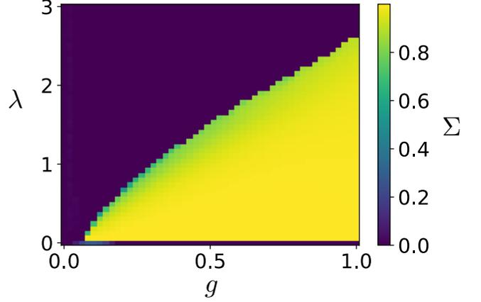
FIG. 8. Correlation coefficient of two reactively-coupled vdP oscillators for  $\Delta = 0.1, r = 1$ .
