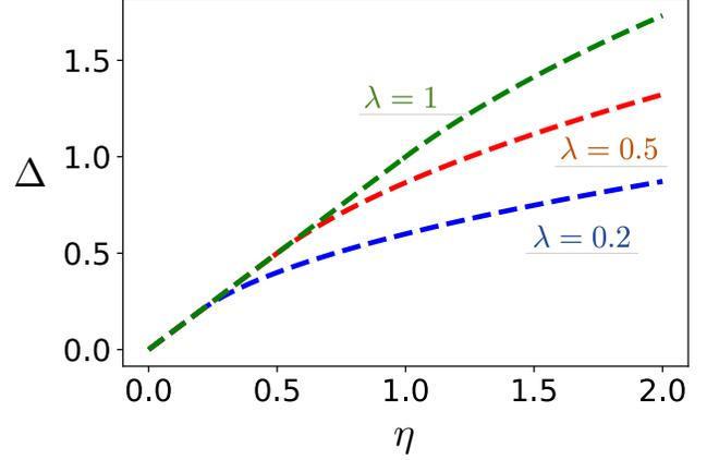
FIG. 6. Synchronization boundaries for different values of  $\lambda$ . The synchronization region lies below the curve in the all cases. The synchronization bandwidth is enlarged as  $\lambda$  is increased for a fixed  $\eta$ .
