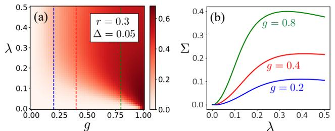
FIG. 3. Positional correlation (8) for two reactively coupled vdP oscillators. (a) Contour of  $\Sigma$  as a function of  $\lambda$  and  $g$  for  $r = 0.3$  and  $\Delta = 0.05$ . The bottom gap of zero correlation agrees with the SL limit. (b) Correlations along the three vertical dashed lines at  $g = 0.2, 0.4$ , and  $0.8$  in subplot (a).
