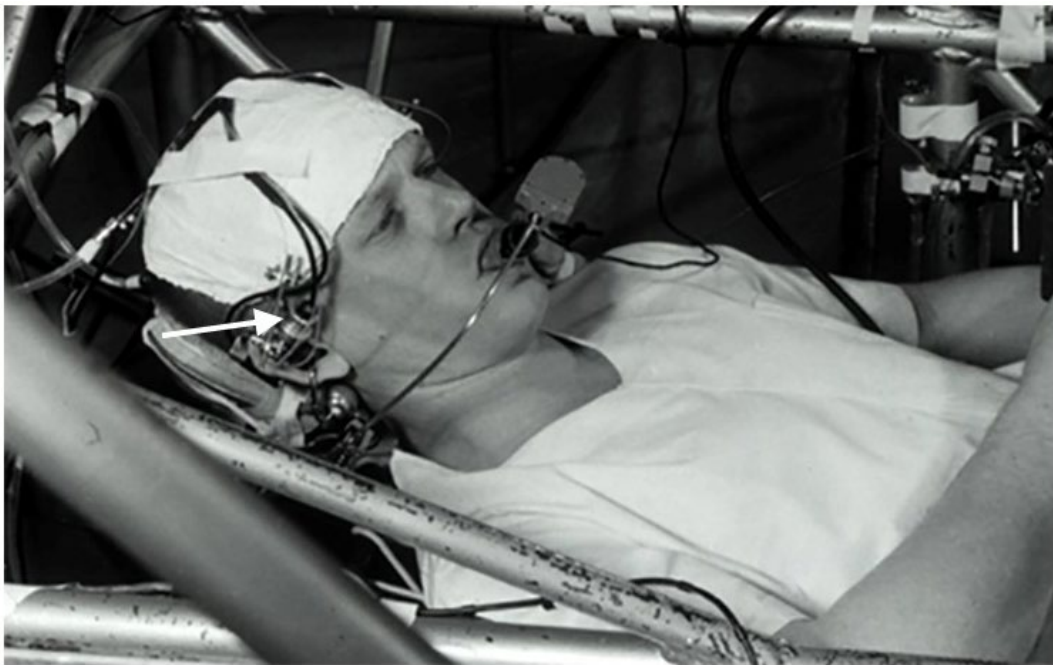
Figure 3: Volunteer in the cockpit of Mayo Clinic’s human centrifuge, wearing earpiece oximeter on right ear, as indicated by white arrow, ca. 1962 (Photo courtesy of Don Hagland). (1954) 3
