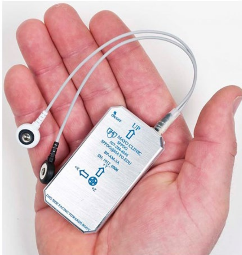
Figure 1. The small battery-powered body-worn units developed for continuous measurement of motion and ECG, worn by the mountain climbers on a Mayo-sponsored expedition to Mount Everest in 2012 [20]. The unit was 38.9 mm wide, 70.2 mm long, 8.9 mm thick; 3 3-axis accelerometers; 2 or 3-electrode, 400 samples/second ECG at 12-bit sampling resolution; 2-week run time. Our goal was to incorporate the analyte measurement capabilities into a physical form factor like these units (this figure also appears in U.S. Patent 8,849,387). (43333) 2
