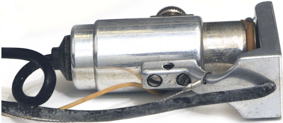
Figure 2: Earpiece oximeter developed at Mayo Clinic, illustrating light and plunger fully depressed against photodetector, ca. 1943. (42175)
