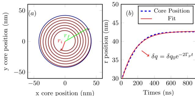
FIG. 3. (Color online). (a) vortex core dynamics affected by amplitude perturbation  $\delta q$ . (b) Core position as a function of time after perturbation, and the fit function that extracts the rate at which the system goes back to the stable trajectory.
