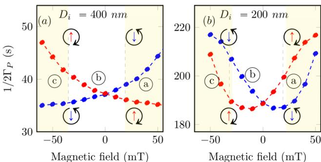
FIG. 4. (Color online). Plots of  $1/(2\Gamma_p)$  as a function of the perpendicular applied magnetic field in regions (a), (b) and (c) for discs of diameters (a) 400 nm and (b) 200 nm, respectively.
