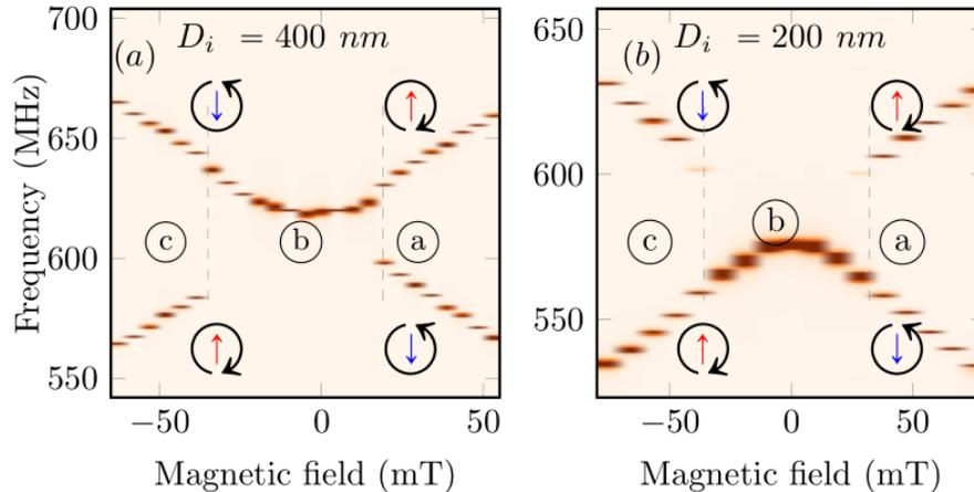
FIG. 2. (Color online). Plots of the coupled STNOs' frequency dependence on the sweeping perpendicular applied field  $H_{\perp}$  between three regions, namely (a), (b) and (c). The plots resemble discs of diameters (a) 400 nm and (b) 200 nm, respectively.
