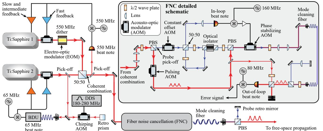
FIG. 2: **Main schematic:** Optical layout for CC, offset-locking, and chirping. The BDU is configured for locking to a fixed 65 MHz beat note. **Inset:** detailed view of the FNC subsystem. The thickness of the lines representing optical paths is used to distinguish high (thick) and low (thin) power beams rather than being an indicator beam waist.
