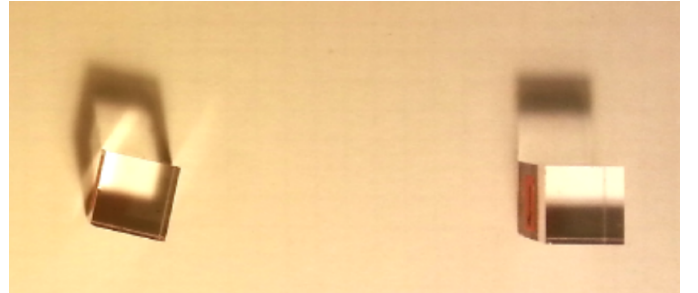
Figure 1: Picture of two cubic 10 \times 10 \times 10\text{ mm}^3 glass samples.
