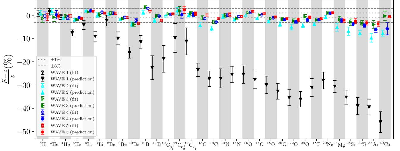
FIG. 7. The plots of deviations between the model outputs and experimental data per nucleon at history matching iterations from WAVE 1 to WAVE 5.
