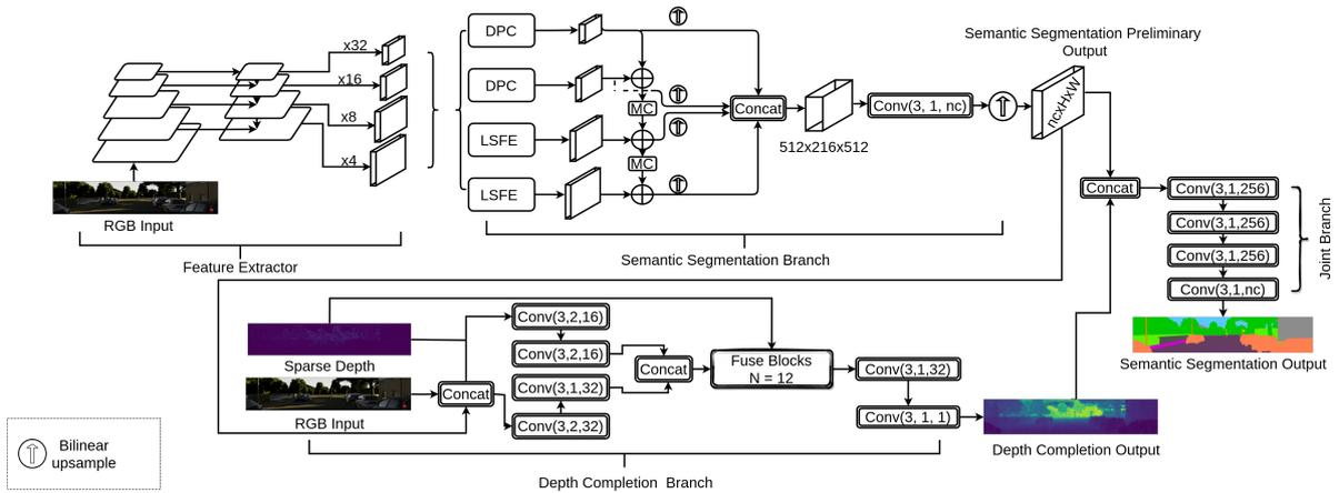
Figure 2: Diagram of the SemSegDepth architecture. The convolutional layers shown in this diagram follow the notation  $\text{Conv}(k,s,c)$  where  $k$  refers to a  $k \times k$  convolutional kernel,  $s$  is the stride, and  $c$  is the number of output feature channels.
