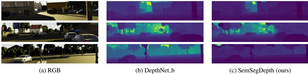
Figure 4: Depth completion results on Virtual KITTI 2. Column *a* shows the RGB image input, column *b* shows the depth completion results using the baseline model DepthNet\_b and column *c* shows the the depth completion results using our model SemSegDepth.
