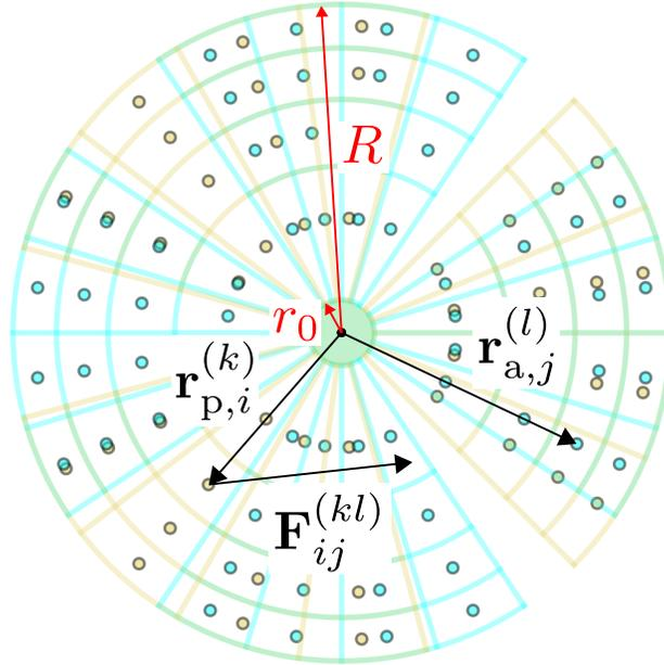
**Figure S1.** Top view of a pendulum with  $N - 1 = 3$  fins suspended above an attractor with  $N = 4$  fins. The vectors  $\mathbf{r}_{p,i}^{(k)}$  and  $\mathbf{r}_{a,j}^{(l)}$  locate the center-of-mass positions of patch  $k$  in pendulum fin  $i$  and patch  $l$  in attractor fin  $j$ , respectively.
