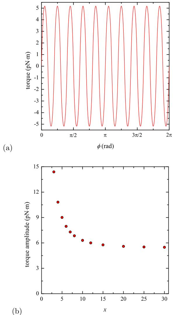
**Figure 4.** The calculated torque as a function of attractor orientation  $\phi$  for a symmetric torsion pendulum with  $N = 10$  fins. For this calculation, each pendulum and attractor fin was subdivided into  $x \times x$  patches, where  $x = 30$ . The torque is periodic in  $\phi$  with the period  $2\pi/N$ . (b) Amplitude of the torque oscillation at the fundamental frequency as a function of  $x$ .
