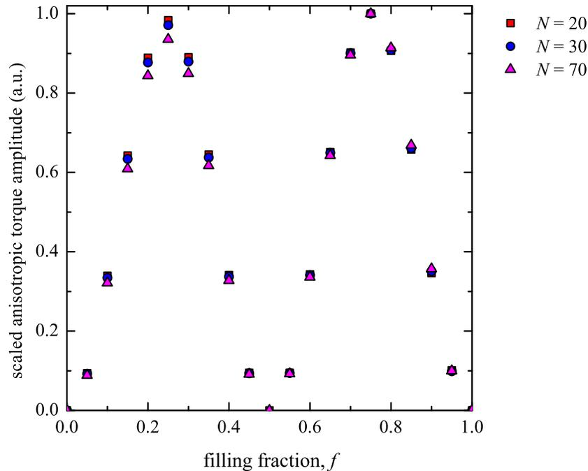
**Figure S2.** Amplitude of the anisotropic component of the torque oscillation as a function of the pendulum and attractor fin filling fraction  $f$ . To facilitate easy comparisons, the data were scaled to make the peak height at  $f = 0.75$  equal to one. Data are shown for  $N = 20, 30,$  and  $70$ .
