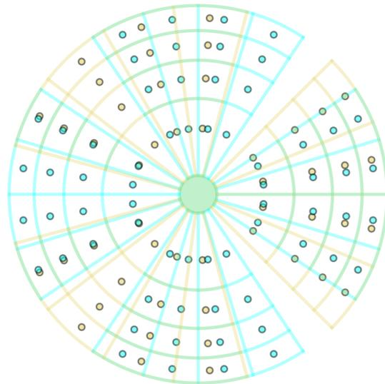
**Figure 3.**  $N - 1 = 3$  pendulum fins (gold) and  $N = 4$  attractor fins (teal) each subdivided into a  $4 \times 4$  grid of patches. The patches of the pendulum fins each have mass  $m_p$  and the attractor patches have mass  $m_a \neq m_p$ . The straight lines along the radial direction and the arc segments define the patch boundaries. The points indicate the centre-of-mass positions of each patch.
