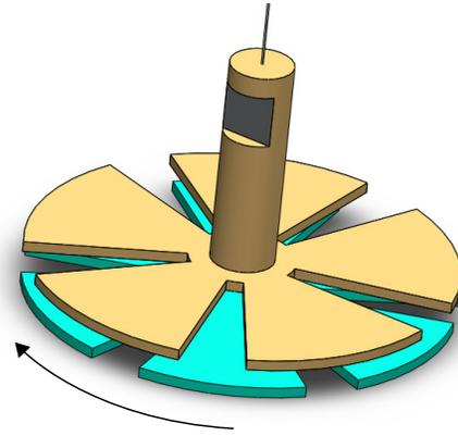
**Figure 1.** Diagram of the proposed experimental setup to test for short-range gravitational anisotropies. In this example, a pendulum (gold) with  $N - 1 = 5$  fins is suspended above an attractor (teal) with  $N = 6$  fins. The attractor rotates at a constant angular velocity beneath the pendulum.
