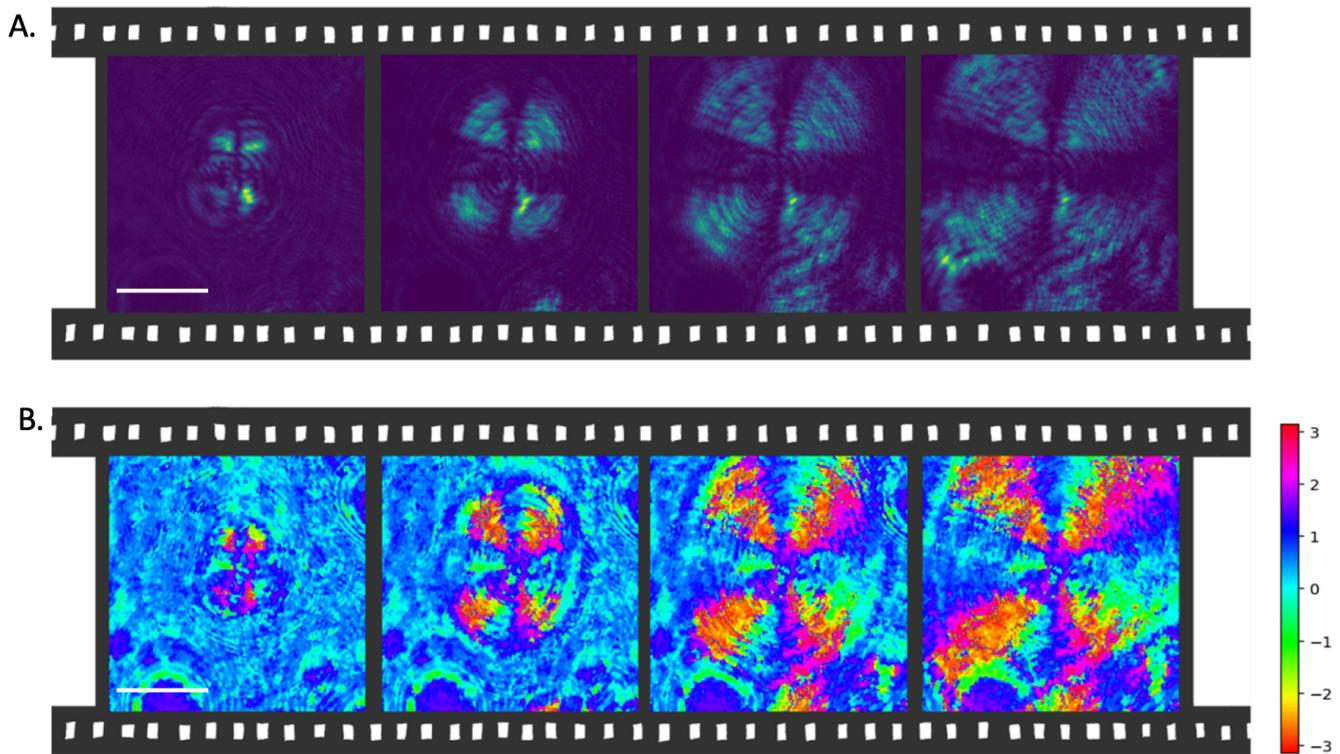
FIG. 4. Frames showing the evolution of polarization distribution during the growth of the sample at  $t=0$ min, 6.5min, 12.8min, 19.1min. The sample was grown at room temperature, from a solution of 10:1 ethanol:water. **a.** Intensity of the beam between cross polarizers at different times during crystal growth. **b.** Plot of the major axis angle of the point by point polarization ellipses at different times during crystal growth. The scale bar corresponds to  $\sim 1$  mm.
