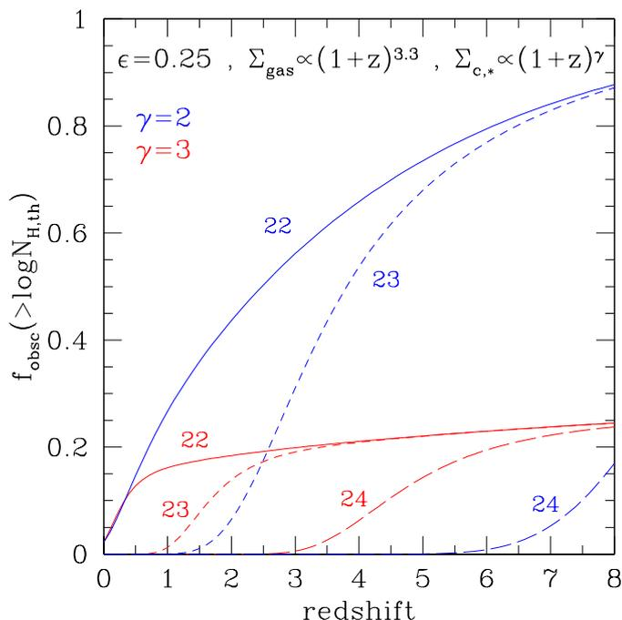
**Fig. 11.** Expected redshift evolution of the ISM-obscured AGN fraction. Blue curves consider a slower ( $\gamma = 2$ ) increase with redshift of the characteristic cloud density  $\Sigma_{c,*}$ . Red curves assume a faster increase ( $\gamma = 3$ ). Labels refer to different thresholds in log column density (see text for details).
