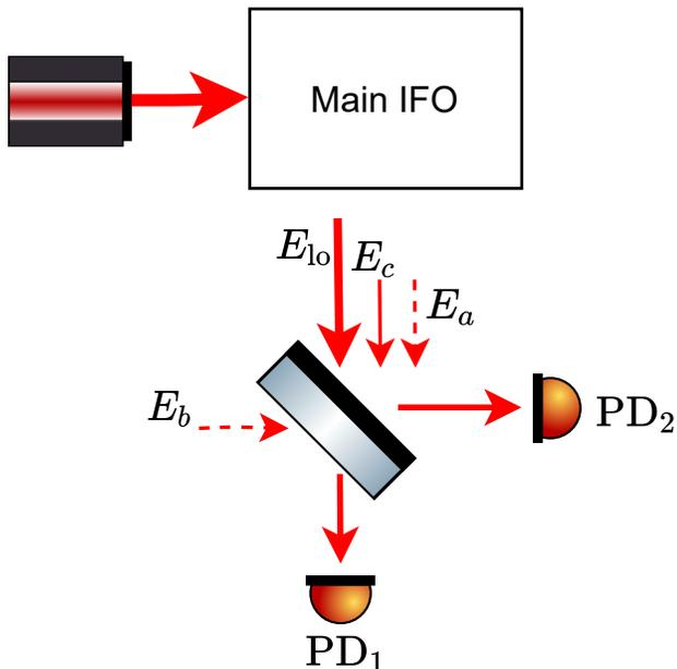
FIG. 1. Cartoon illustrating the readout port of an aLIGO-like GW detector.
