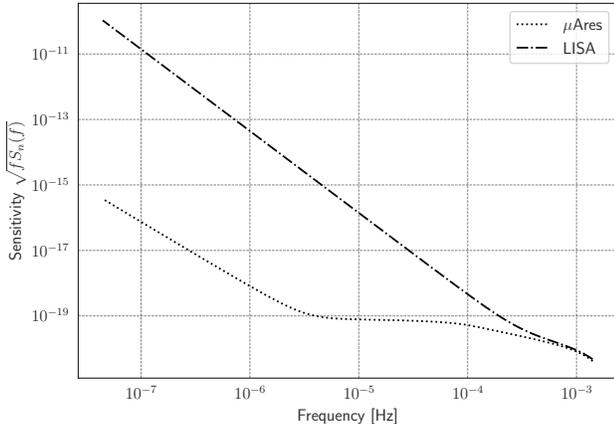
FIG. 3: Sensitivities for LISA (dot-dashed line) and  $\mu$ Ares (dotted line) in the relevant frequency range.
