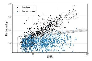
FIG. 3. The test samples plotted in the SNR- $\chi^2$  plane after training is complete. Lines of constant re-weighted SNR are plotted. We can see that at high SNR values there is good separation between the noise samples (black dots) and signal samples (blue triangles), allowing the model to down-weight noise triggers heavily.
