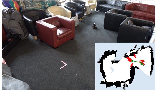
Fig. 1: A small compute-constrained mobile robot exploring an office environment, overlaid with its built occupancy map. Our proposed method uses the map to generate an informed distribution viewpoints (red arrows), capturing the inherently multi-modal nature of exploration planning reflecting the regions of gray unknown space. It identifies the NBV (green) to quickly explore the scene.
