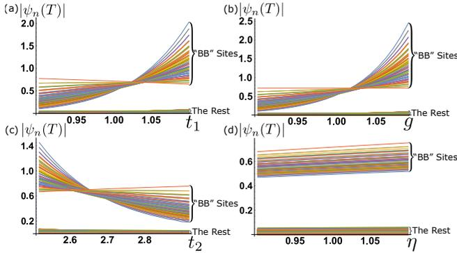
FIG. 8. Performance of 2D laser array with other system parameters, in terms of saturated magnitudes of the state amplitudes on each site,  $|\psi_n(T)|$ , with varying intracell couplings  $t_1$  (a), the strength of the non-reciprocal hopping parameter  $g$  (b), intercell couplings  $t_2$  (c) and nonlinearity  $\eta$  (d). Unless specified otherwise, parameters are chosen the same as Fig. 7.
