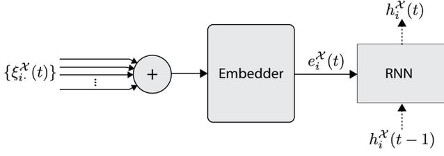
Fig. 4: An illustration of the EdgeRNN structure.
