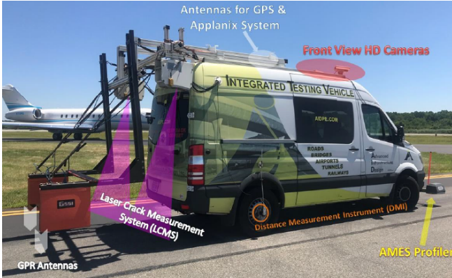
Figure 1: Example of specialized road distress measurement vehicle, developed by Advanced Infrastructure Design Inc. , showcased in [6]
