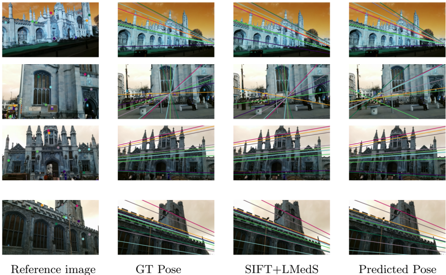
Fig. 2. Qualitative evaluation of epipolar lines for corresponding key-points of reference images, as represented by same colour of lines. First column represents the reference images with keypoints. Second, third, and fourth column represents epipolar lines based on, ground truth pose, SIFT+LMedS, and proposed RelMobnet
