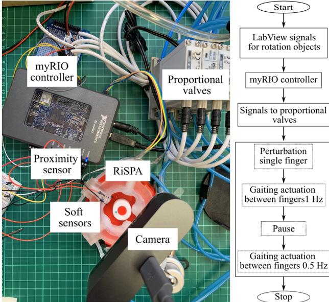
Fig. 3. The experimental setup for characterising the soft sensors and tracking the rotation of the manipulated object and experimental architecture.
