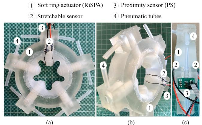
Fig. 2. Soft ring actuator with three sensors installed, 2 soft sensors and one proximity sensor. The soft sensors are attached to the cap of the soft finger.
