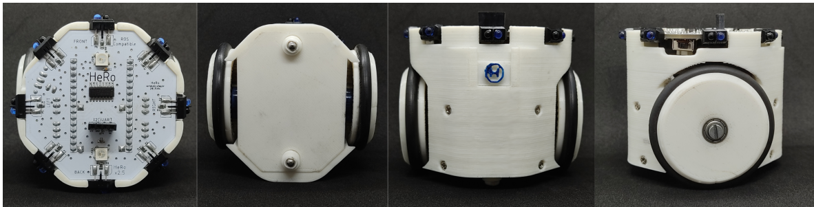
Fig. 6: Top, bottom, front, and left views of the HeRo swarm platform.
