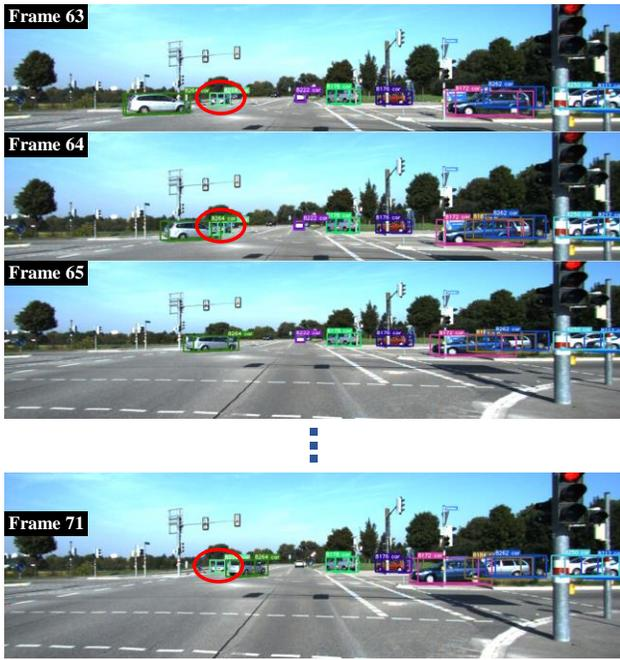
Fig. 4. Qualitative Evaluation - An example using sequence 0010 in the testing set where our method maintains the original trajectory without incurring IDSW, when the vehicle is blocked for several consecutive frames and then reappears in the sensor FOV.
