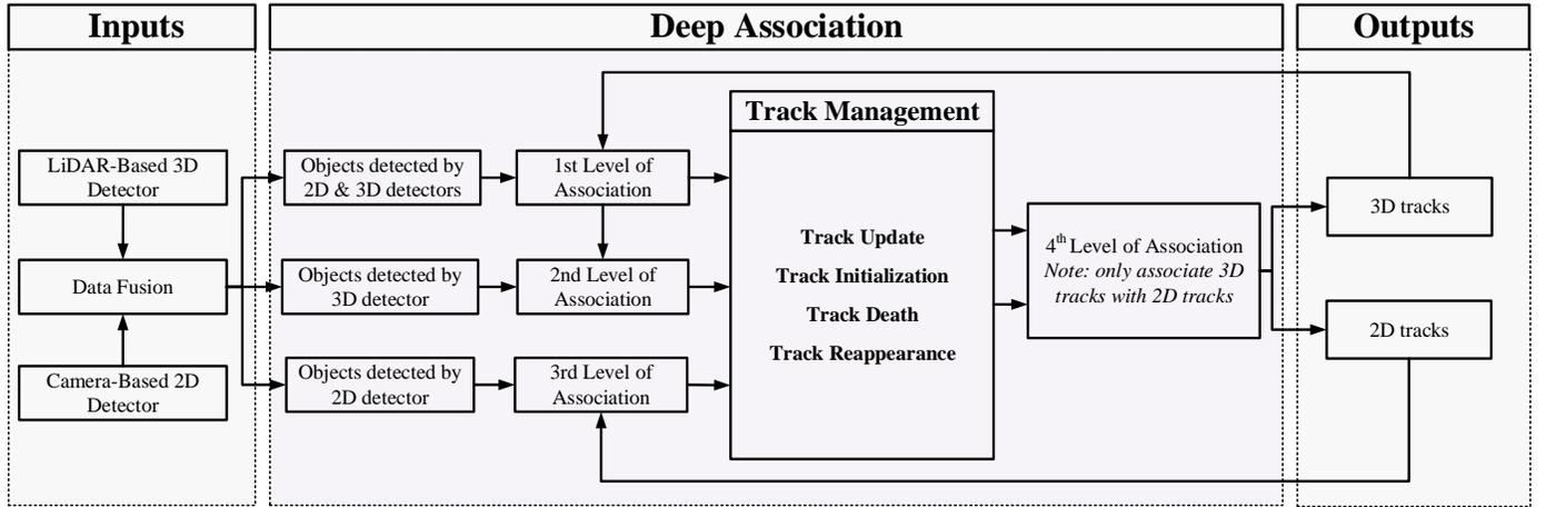
Fig. 2. The system architecture of the proposed camera-LiDAR fusion-based method.
