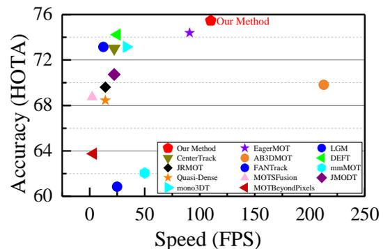
**Fig. 1.** MOT performance of the proposed method on the KITTI 2D MOT leaderboard with relation to several baseline trackers. The higher and the more rightwards, the better. Our method achieves an optimal HOTA and a very high speed.
