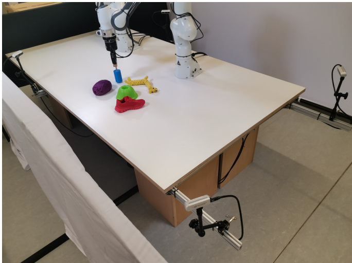
Figure 16: Setup of real world experiments. 4 camera views from the side. No top down view.
