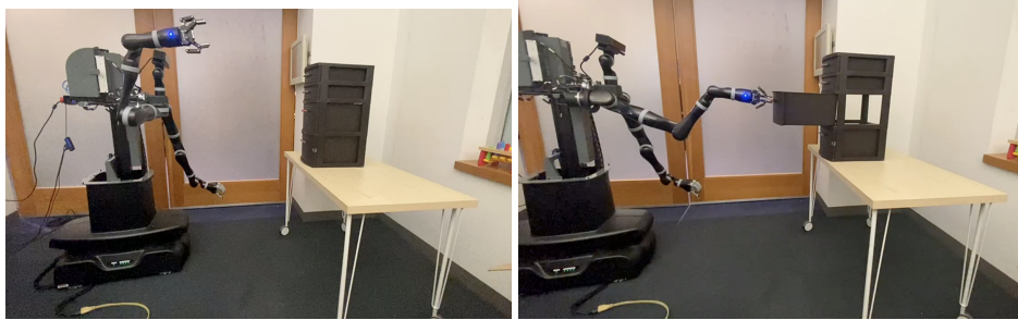
Figure 2: Kinova Movo opening a drawer using the drawer opening policy from ManiSkill
