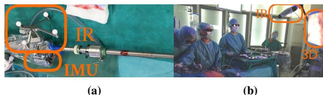
**Fig. 1: Data Acquisition (a) IMU sensorboards and IR passive targets attached to stereoscopic laparoscopic camera (b) IR sensor and 3D monitor in the operatingroom**
