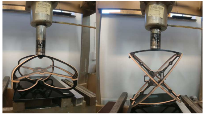
Fig. 4. Hydraulic press test experimental setup for case (iii) and (iv).
