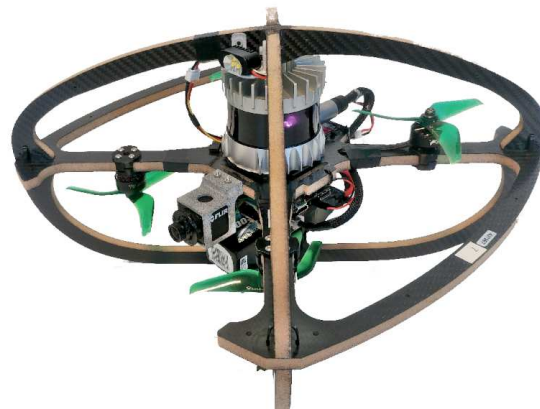
Fig. 1. RMF-Owl: The collision-tolerant flying system designed for resilient autonomous subterranean exploration.
