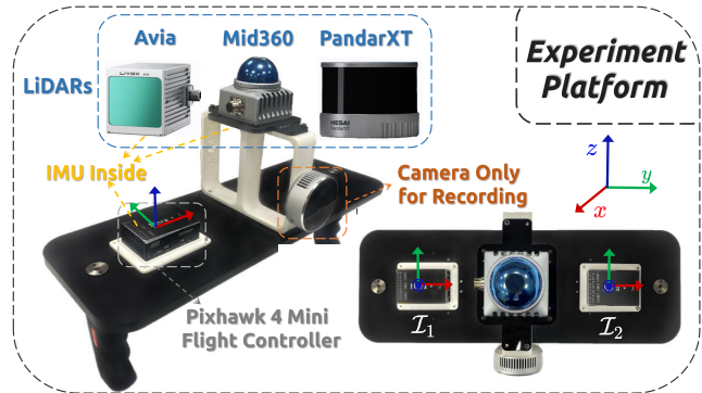
Fig. 1. Experiment platform including multiple LiDARs (Non-repetitive scanning Livox Mid360, mechanical spinning Hesai PandarXT, small FoV Livox Avia) and built-in IMUs of LiDARs and Pixhawk flight controller. RealSense L515 camera is only used for recording videos in first personal view.
