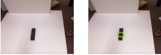
Fig. 7 Hand labelled positive grasp rectangle is drawn on an object for creating the paired-image dataset. The gripper plates orientation is shown by green sides of the grasping rectangle.
