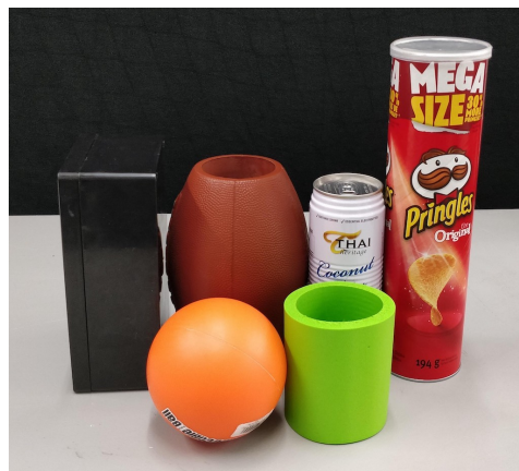
Fig. 7. Objects used for our robot experiments. From left to right, the objects and surface properties are: plastic box (planar, smooth, rigid), plastic ball (spherical, smooth, rigid), football sleeve (spherical, rough, deformable), foam sleeve (cylindrical, smooth, deformable), metal can (cylindrical, rough, rigid), and cardboard can (cylindrical, smooth, rigid).
