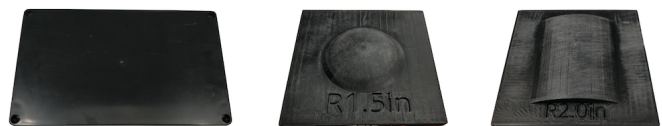
Fig. 4. Surfaces used for slip data acquisition, from left to right: a planar box lid, a spherical plastic surface (radius 1.5 in), and a cylindrical plastic surface (radius 2 in). The latter two surfaces were 3D printed and sanded to remove irregular edges.
