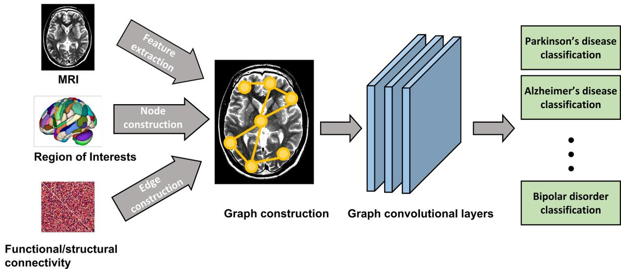
**Fig. 3. The framework of developing GCNs in neuro-imaging analysis. Multi-modality MRIs are firstly converted into graph structure which is determined by the region of interest in terms of real human brain signals or fiber connectivity (e.g., node and edge definitions). Through graph-level model development and inference, we highlight numerous image-based analysis and diagnosis of diseases in neurology.**
