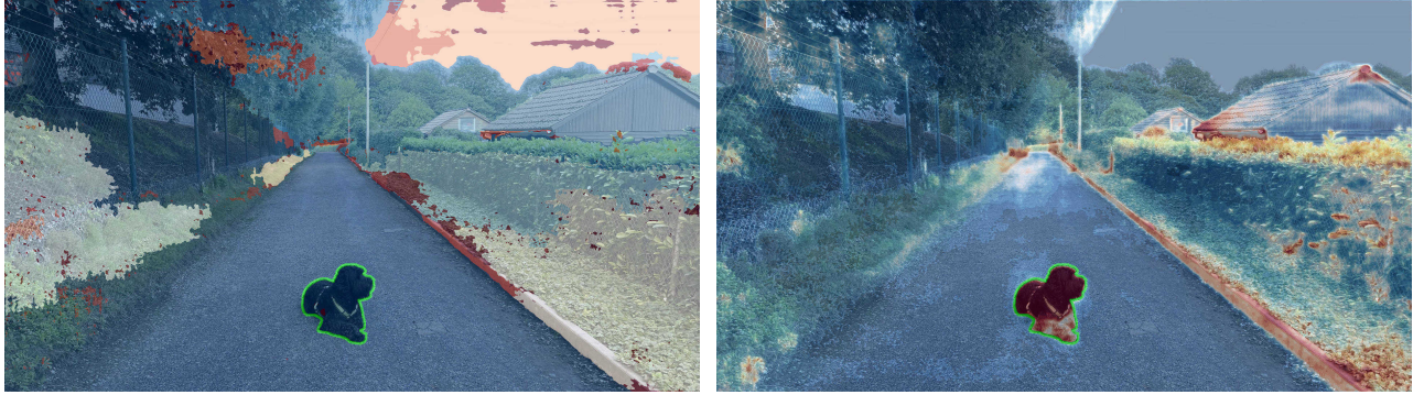
Fig. 7. A comparison of anomaly scores obtained by meta classification (left) and entropy (right) on an image from RoadObstacle21. The dog on the image is the anomaly of interest (indicated by green contours), which would have been overlooked by meta classification but entirely detected by the entropy.
