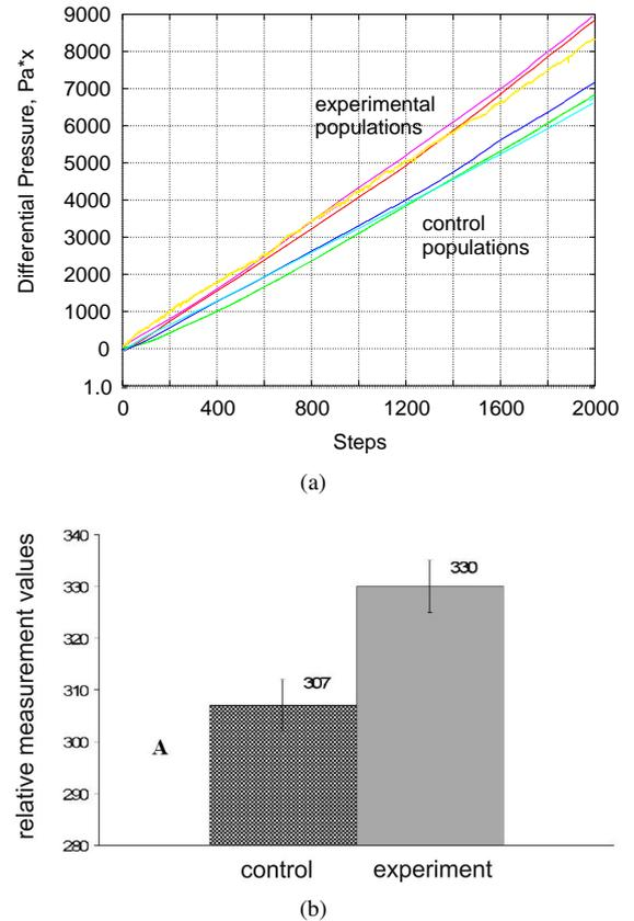
Fig. 1. Examples of measurements from previous versions of pressure sensing system, yeast are exposed by WES [50], the difference in pressure of experimental and control populations is well visible: (a) (Stuttgart) 6-channels pressure sensing system based on the Murata SCP1000-D11 sensors, images from [26]; (b) (Orel) 15-channels pressure sensing system, image from [12].
