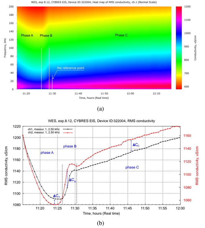
Fig. 3. Electrochemical phases of fermentation dynamics: (a) EIS data (3D multi-frequency representation) from the channel 1, the phase A – sedimentation process, the phase B – fast dynamics, the phase C – slow dynamics; (b) 2D plot at 2.5 kHz of the channels 1 and 2 from (a), the channel 2 is impacted by WES, different EIS dynamics of impacted and non-impacted channels is well visible in all phases of fermentation process.
