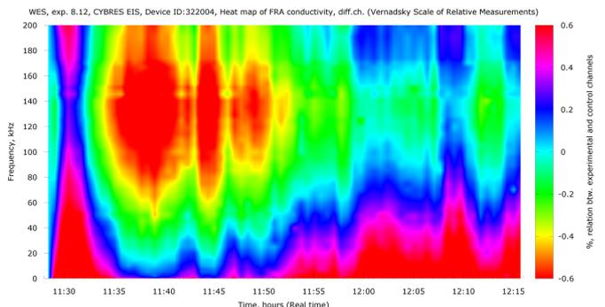
Fig. 15. EIS dynamics from Fig. 3, the set point is selected at the transition between phases B and C. The appearing time-frequency patterns can be used for identification of chemical and biological processes in these phases.
