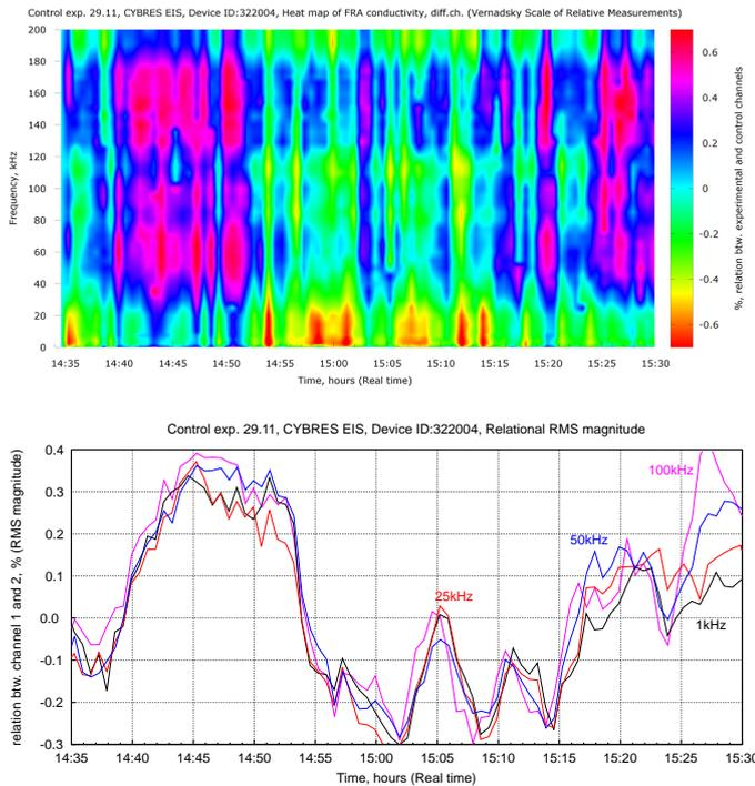
Fig. 7. (a) EIS dynamics of the control attempt without any impact, the reference point is selected in the way shown in Fig. 3(a); (b) 2D plot at 1 kHz–100 kHz, the variation is about  $\pm 0.4\%$  (origin shifted to zero).
