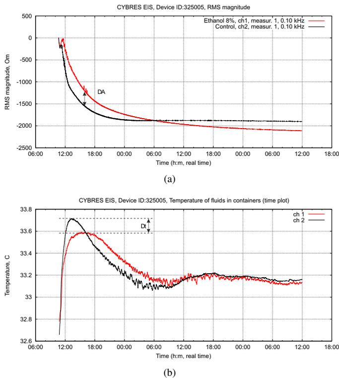
Fig. 9. Long-term yeast fermentation EIS dynamics at 0.1 kHz with 8% Ethanol in Ch1. (a) RMS magnitude; (b) Fluids temperature in containers.
