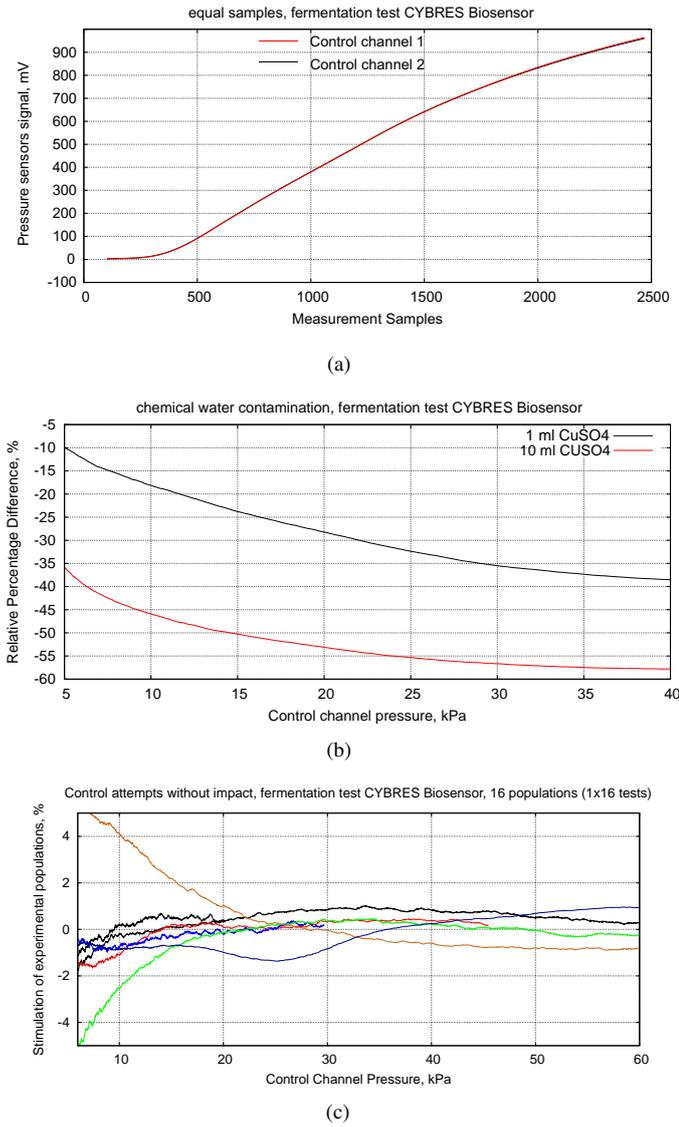
Fig. 6. (a) Control attempt with equal conditions for both populations (equal samples); (b) Example of chemical water contamination –  $CuSO_4$  is added to the yeast solution in the experimental channel. Each curve represents an averaging of 8 pressure sensing channels, the x-axis represents measurement samples (about 2 s); (c) Repeated control measurements with equal conditions for both populations.
