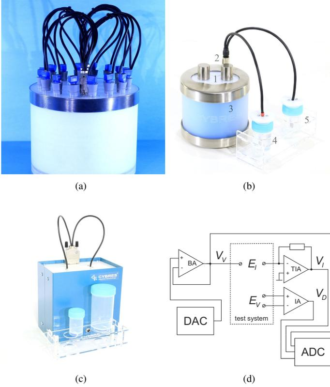
Fig. 2. (a) The 16-channel pressure sensing system; (b) The differential EIS spectrometer with temperature stabilization of samples and electronic components; (c) Adapted version of the EIS device with 100 ml containers for the biosensor purposes; (d) Structure of one EIS measurement channel, see description in text.
