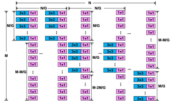
Fig. 2. Structural layout of dual convolution.
