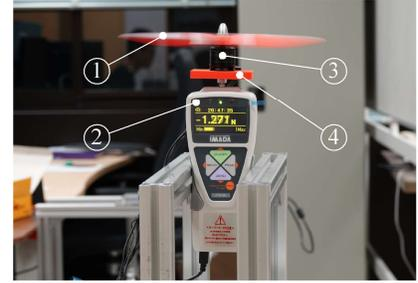
(a) Thrust force measurement experiment
