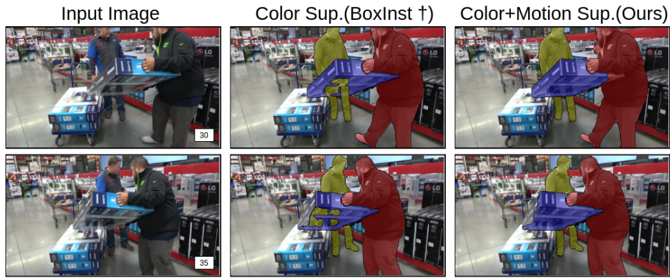
Figure 9: A qualitative comparison between baseline(color only) and our method. The baseline model predicts an erroneous mask for the distant man due to color similarity with reflection on the TV case. While the inclusion of motion alleviates this in our method.
