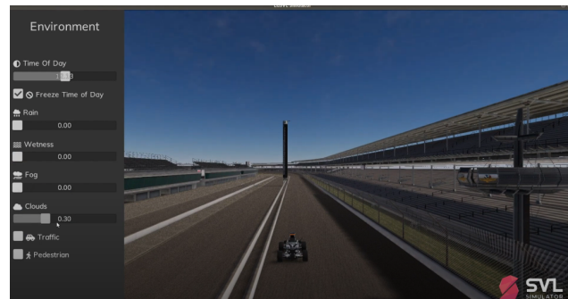
Fig. 11. F1TENTH vehicle in the SVL simulator [73] on a 1:10 scale version of the Indianapolis Motor Speedway.
