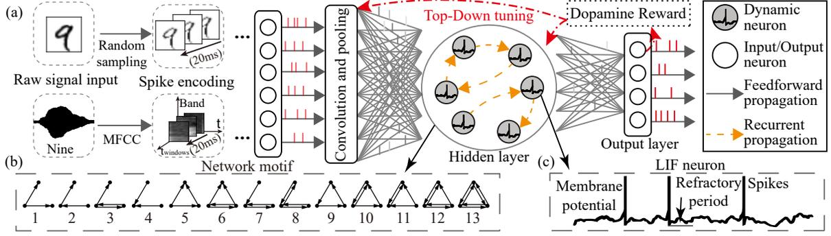
**Fig. 1.** The architecture of MR-SNN. (a) The architecture of MR-SNN on the multi-sensory integration task. (b) The example of artificial 3-node Motifs. (c) The spiking neuron with dynamic membrane potential.
