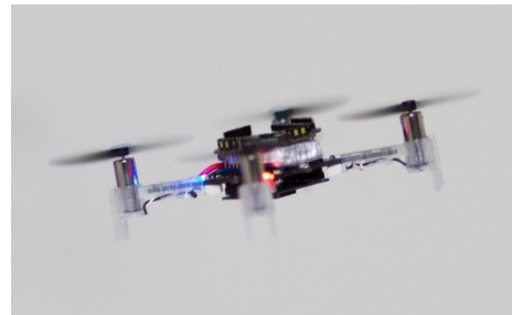
Fig. 9. Crazyflie, a 39-gram MAV from company Bitcraze.
