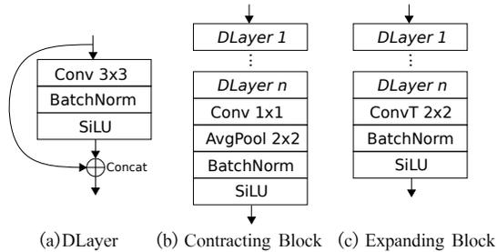
Fig. 3: Configuration of each block in the DenseNet-based autoencoder for keypoints extraction. Each block contains 3 or 4 layers, the convolutional dilation increases accordingly in each layer.
