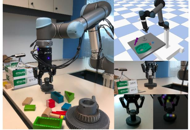
Fig. 1: End-to-end RL of robotic manipulation with keypoints representation in simulation and real-world
