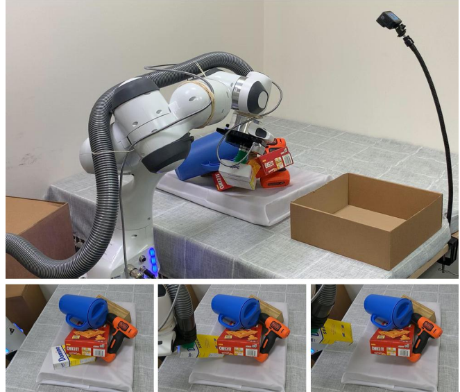
Fig. 1: SafePicking extracts target objects with minimum destruction by generating a safe end-effector trajectory given a raw depth observation and object poses from an object-level map.
