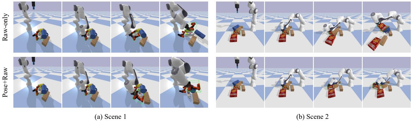
Fig. 4: Qualitative results of the model ablation , in which we compare Raw-only , which uses only a heightmap observation, and our full model Pose+Raw , which uses object poses along with a heightmap.
