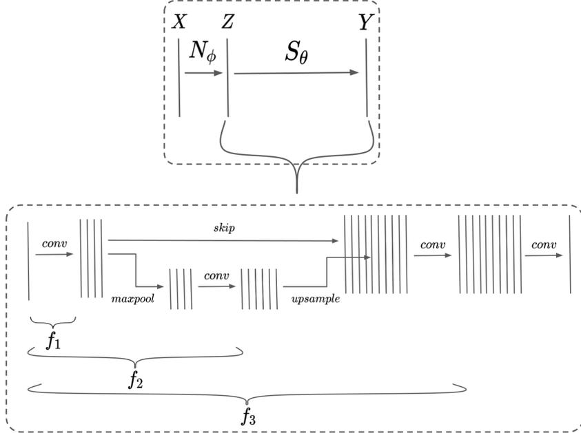
Figure 2: Representative schematic of a test-time adaptable CNN.
