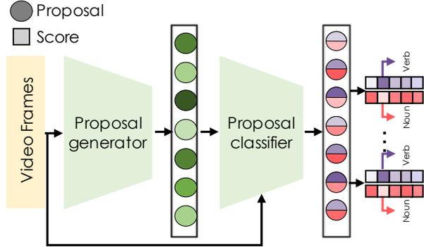
Figure 2. **Separate-stage framework for temporal action localization.** Proposal generation: given a sequence of snippet features, action proposals with start/end timestamps are produced. Proposal classifier: given a set of proposal features, classification scores for each proposal are produced.
