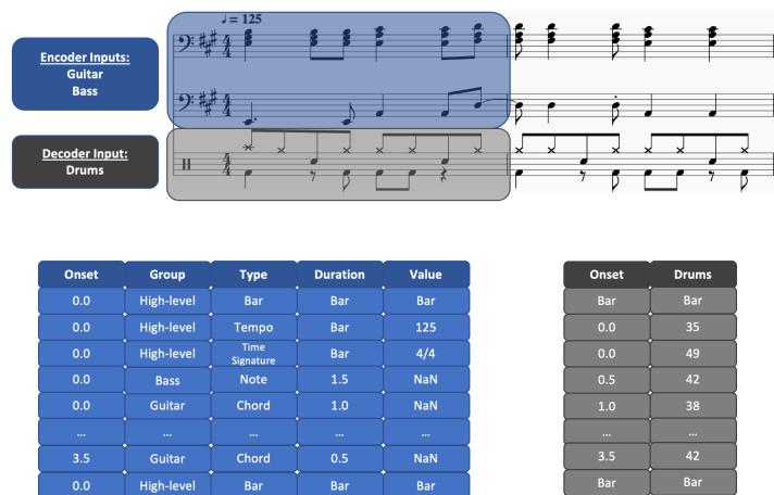
Fig. 1. Illustrated example of a training snippet represented in the proposed CP-based representation (for Encoder and Decoder inputs).
