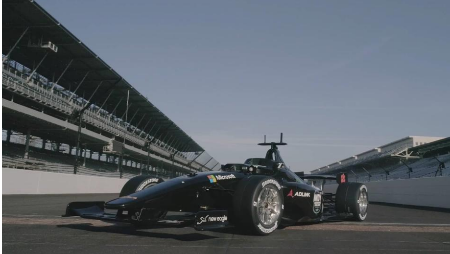
Figure 3: The autonomous Dallara - AV21 racecar for the Indy Autonomous Challenge [36]
