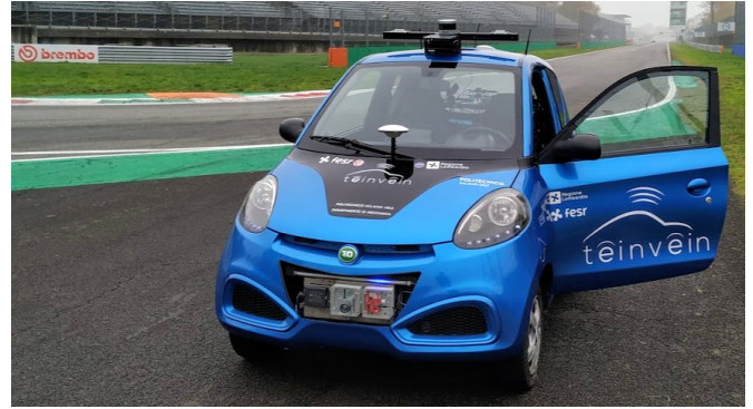
Fig. 1: Image of the experimental vehicle (Ego Vehicle) instrumented with Lidar, Radar and Camera employed for the dataset acquisition and algorithm validation
